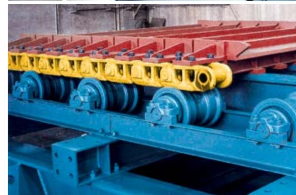
Apron feeders are designed for conveying capacities of more than 14,000 t/h and can be integrated into stationary, semi-mobile or mobile plants.
