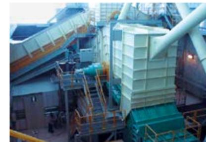
As all drives can be set accurately, it is possible to combine two or three apron feeders, thus allowing the material for cement production to be pre-homogenized.
