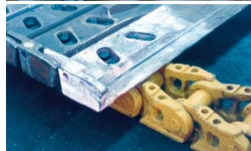
Cast aprons checked for surface cracks
