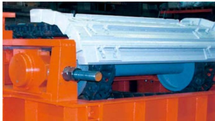
The chain tension can be adjusted via tensioning spindles. In combination with the relocatable drive shaft, it ensures optimization of the feeder discharge point, e.g. into the crusher.
